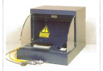
Test cabinet for HV testing.
