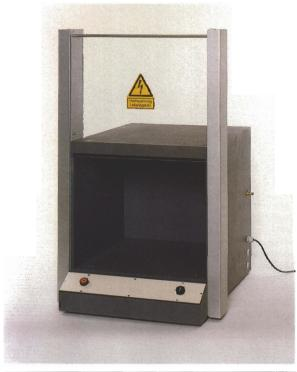
The all-welded plastic enclosure permits tests up to 8 kV AC or 12 kV/DC. The protective door runs in ball-bearings and is pneumatically operated. For tests assessed with "Pass", the protective door opens automatically. In the event of a fault, an acknowledgement key must be actuated. A maintenance unit with compressed-air connection (minimum 5 bar) is installed at the rear. The test chamber is prepared for connection to ELABO high-voltage testers 2GA27 90-1... as standard.
